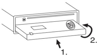
If the device was still switched on when you detached the control panel, it will automatically switch on with the last setting activated (radio, CD, CD changer or AUX) when the panel is replaced.
