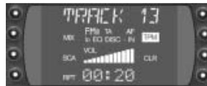
Use the corresponding softkeys to select MIX, SCAN, RPT (Repeat) and TPM in CD and changer operation.
