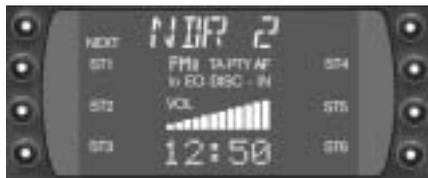
Press **DIS** for approx. 2 seconds: Display will alternate between the clock and the waveband (incl. the memory level for FM).
