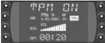
If “TPM” is highlighted in the display, this means that TPM playback is active. All of the tracks on the CD stored in this operating mode will be played. If you activate SCA (scan) as well, these tracks will be scanned.
